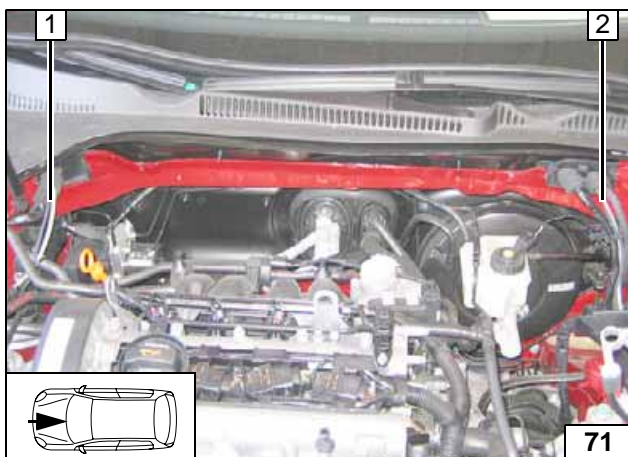
1 Wiring harness of metering pump, fuel line
